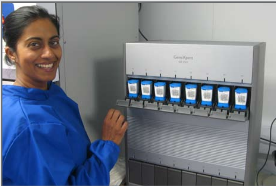
Figure 6. Sharmila Naidoo showing a typical batch being run on the Xpert® MTB/RIF.
